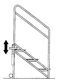
**Step 2**Tip the stairway as needed to fit the hooks under the frame of the platform.
